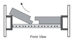
4) Important: push both baffle bricks so they are tight against the side walls.
